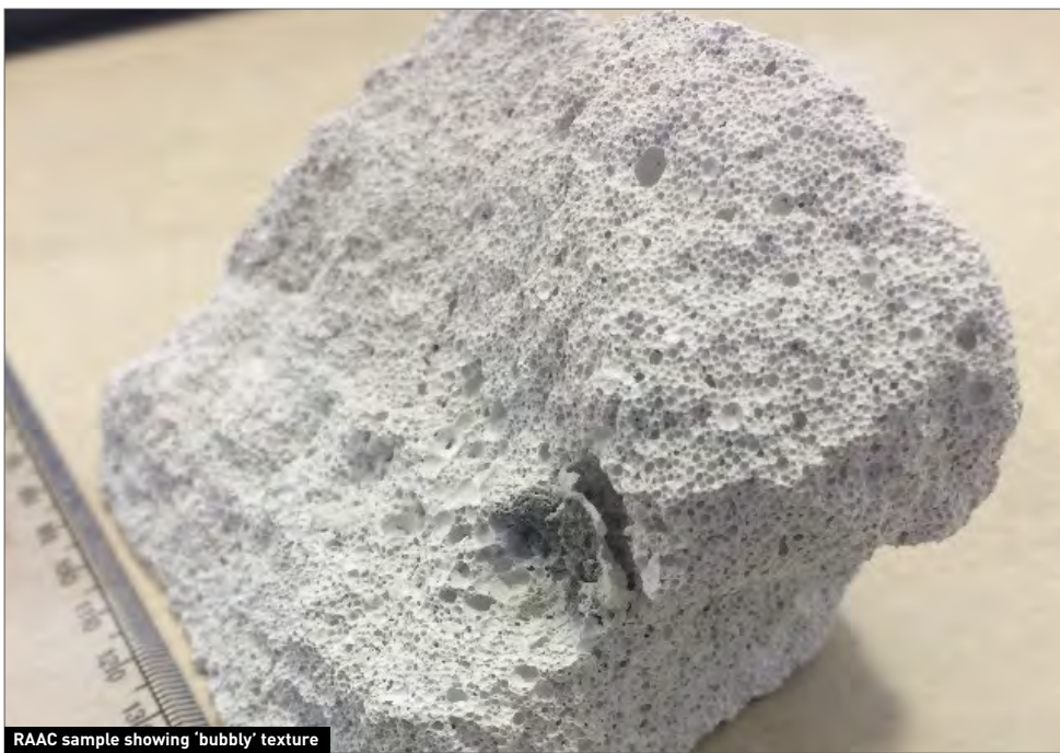
RAAC sample showing 'bubbly' texture
